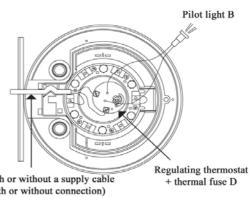
With or without a supply cable (with or without connection) according to the sample
