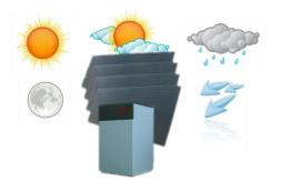
The temperature difference brought about by the previous factors ensures that the fluid will change to vapour state inside the panel.
